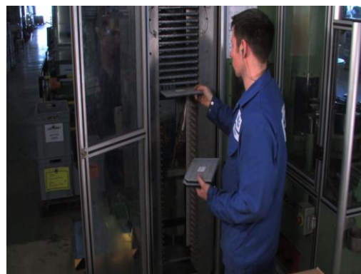
Charging of filled magazines into the primer inserting machines
